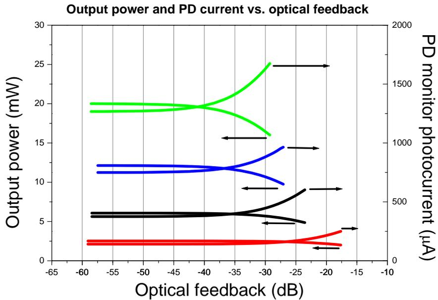
Fig.5. Results on study of SLD-371 reaction to optical feedback. red: SLD-371-MP, black : SLD-371-HP1, blue – SLD-371-HP2, green – SLD-371-HP3.
